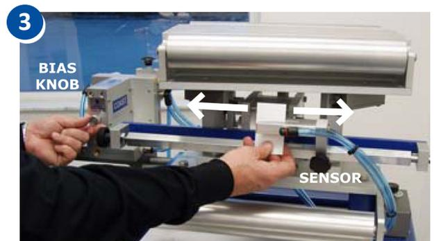
There is an interrelationship between the air pressure, needle valve, and bias adjustment knob, and when adjusting one, you may have to slightly readjust the other. Once the system is properly set, it will move smoothly and responsively with a balanced shifting speed. Further adjustments should not be needed.
